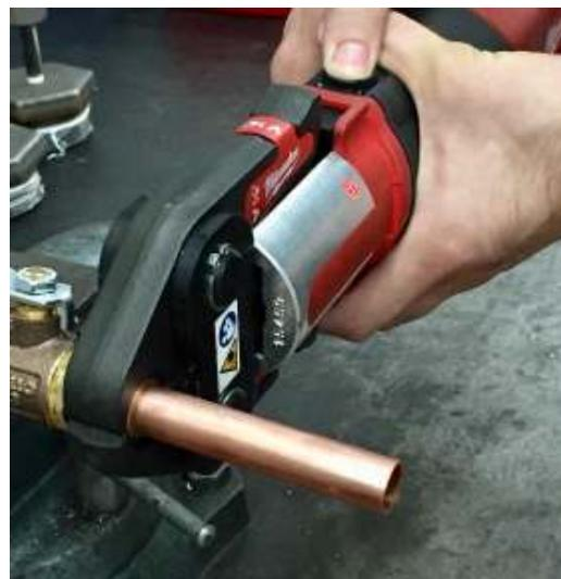
*Warning: To avoid pinch point injury, keep hands and fingers away from jaws. Avoid sharp edges that may have formed on the valves during the pressing operation.*
