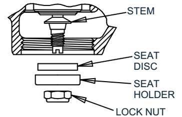
**CAUTION:** Always relieve the spring pressure by unscrewing the adjusting screw before attempting to unscrew the cap assembly.
