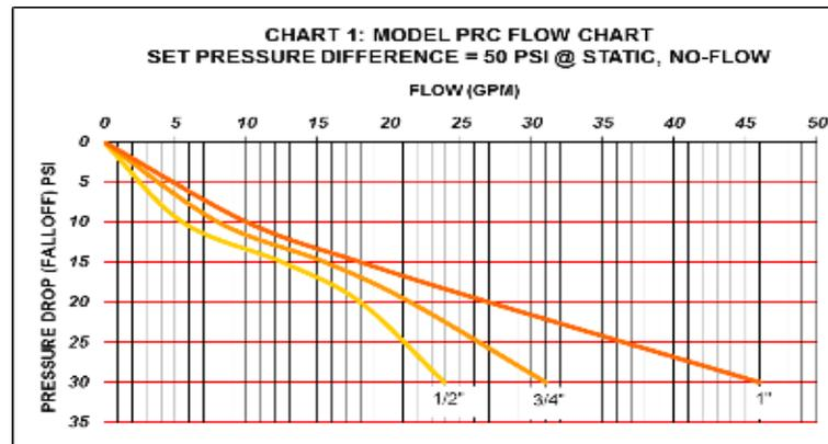
NOTE: Although this chart shows curves at a 50 psi set differential, curves for other settings are similar. The curve shifts slightly to the left for a smaller differential and to the right for a greater differential.
